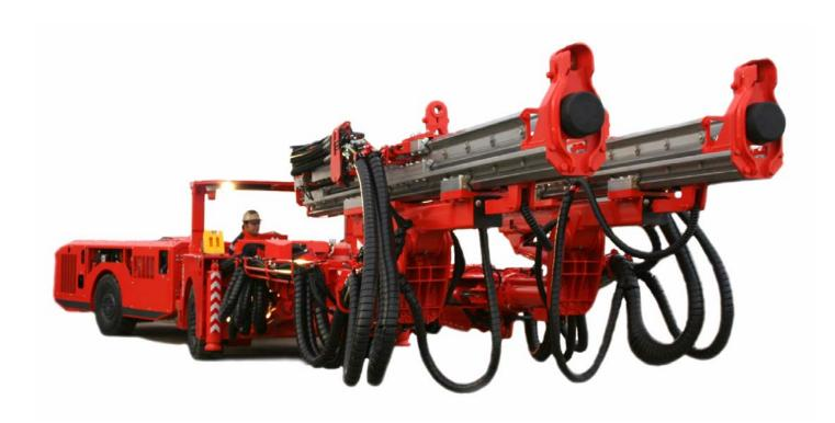
Sandvik DD220L is a low profile twin boom electrohydraulic drilling machine designed to work in excavations with headroom as low as 1.7 m.
