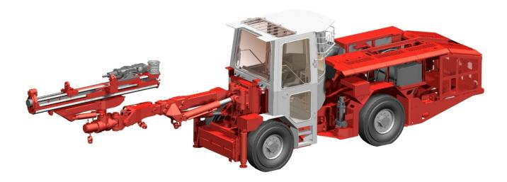
Sandvik DD311D-40EC is a single boom electro-hydraulic jumbo with the ability to drill on both diesel and electric power. It is designed for fast and accurate drilling in drifting and tunneling of 40 m² cross sections. The hydraulic controls enable accurate and efficient drilling performance.
