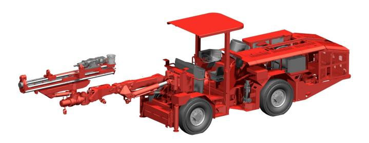
Sandvik DD311D-40E is a single boom electro-hydraulic jumbo with the ability to drill on both diesel and electric power. It is designed for fast and accurate drilling in drifting and tunneling of 40 m² cross sections. The hydraulic controls enable accurate and efficient drilling performance.
