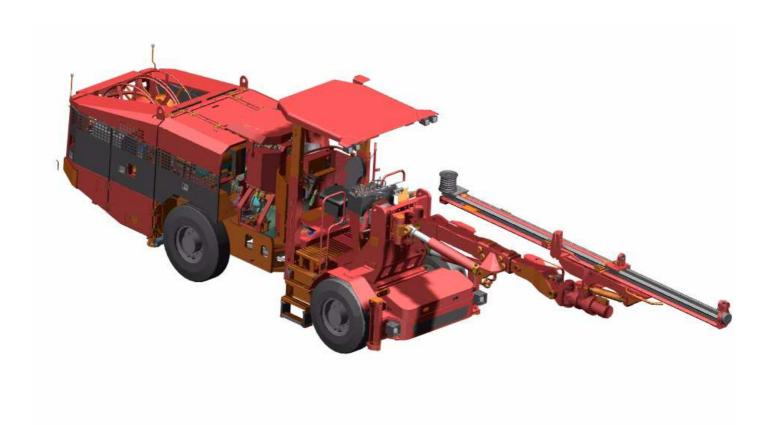
The Sandvik DD411-60 is a single boom electrohydraulic jumbo for fast and accurate drilling in drifting and tunneling of up to 54m<sup>2</sup> cross sections.
